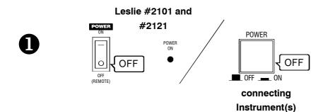
Make sure the power on the Leslie Speakers as well as on the connecting instrument(s) is "OFF."
