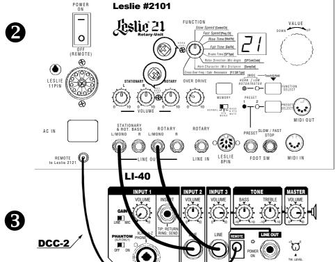
Make the connection shown in the figure at the left. Connect the Rotary-Unit to the Stationary-Unit using the DCC-2 Cable. Then connect the sound source to the LINE IN jacks as shown. Finally, connect the Stationary-Unit to AC power.
